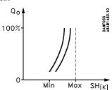
Regulation is here based on the evaporator's load by means of MSS search (MSS = lowest permissible superheat).
